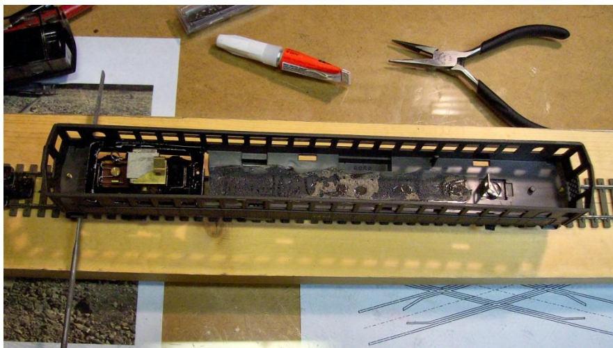
Supported at proper height for gluing
